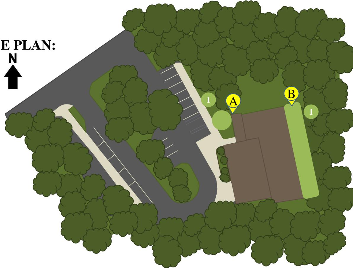
**1 BIORETENTION SYSTEM:** Bioretention systems could be installed at the northern corner and along the eastern side of the library. A bioretention system will reduce runoff and allow stormwater infiltration, decreasing the amount of contaminants that reaches catch basins.
