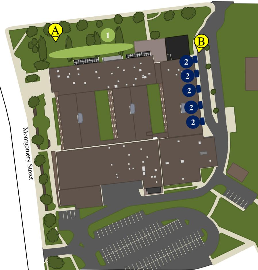
**1 BIORETENTION SYSTEM:** A bioretention system could be installed along the northern side of the building after disconnecting downspouts. A bioretention system will reduce runoff and allow stormwater infiltration, decreasing the amount of contaminants that reaches catch basins.
